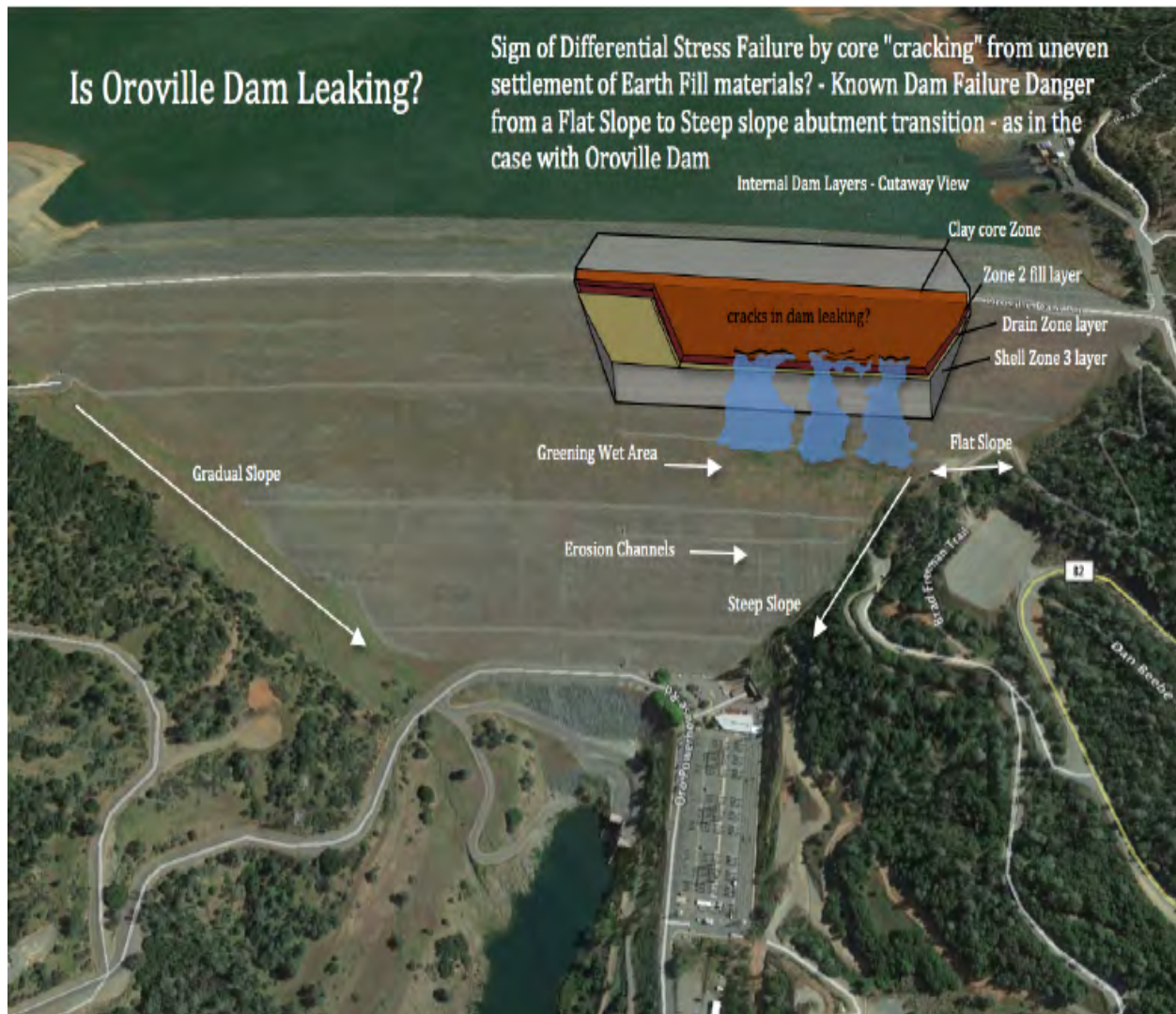
Figure 3: Does the water 'seepage' in the Oroville Dam endanger its Safety and Reliability?
