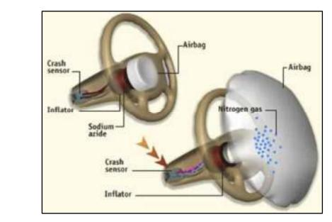
81. The Defective Inflators—which are equipped in both driver—and passenger-side airbags—are toroidal stored gas hybrid inflators, which means they are shaped like a small, circular can (toroidal) and comprised mostly of highly compressed gas, with a secondary chemical compound propellant used to heat the stored gas so that it expands enough to sufficiently fill the
