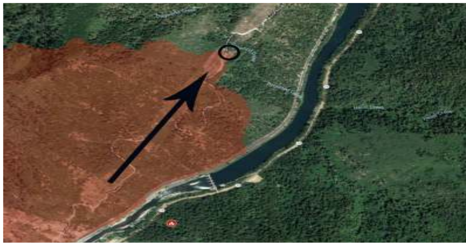
18 19 The Black Arrow Follows the Path of PG&E Transmission Lines with the Black Circle Depicting the Suspected Area of Origin of the Camp Fire 14
