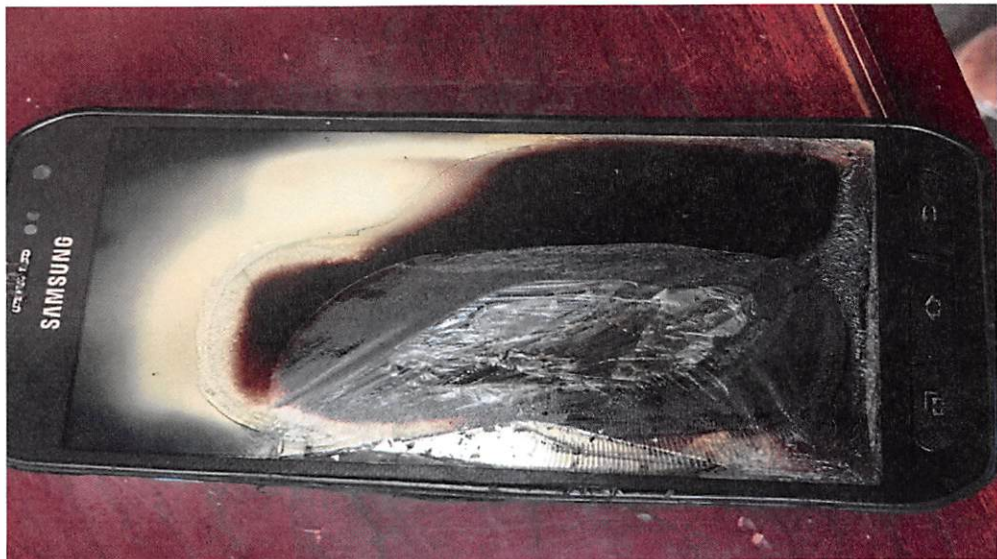
27 Front of BRANDON ’s Galaxy S6 Active smartphone following explosion.
