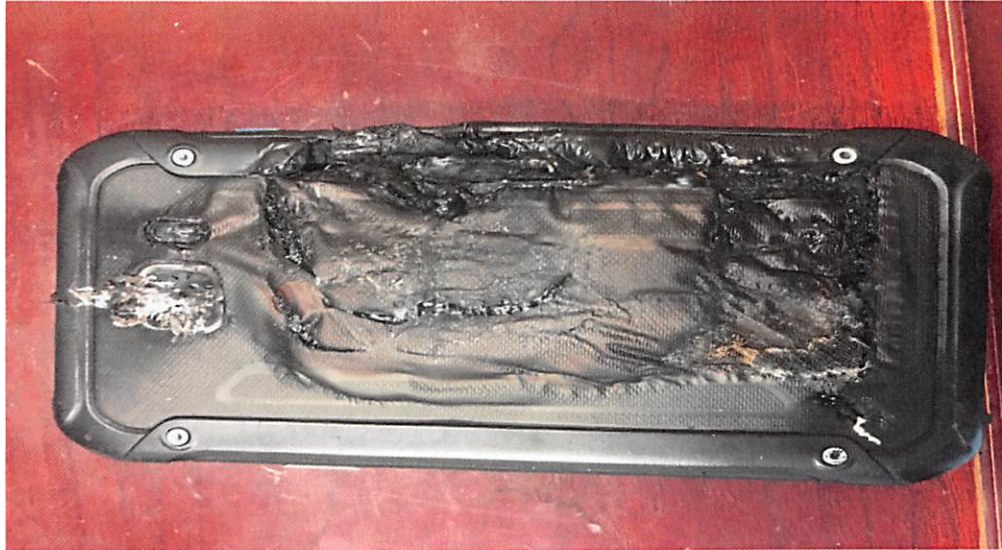
Rear of BRANDON’s Galaxy S6 Active smartphone following explosion.
